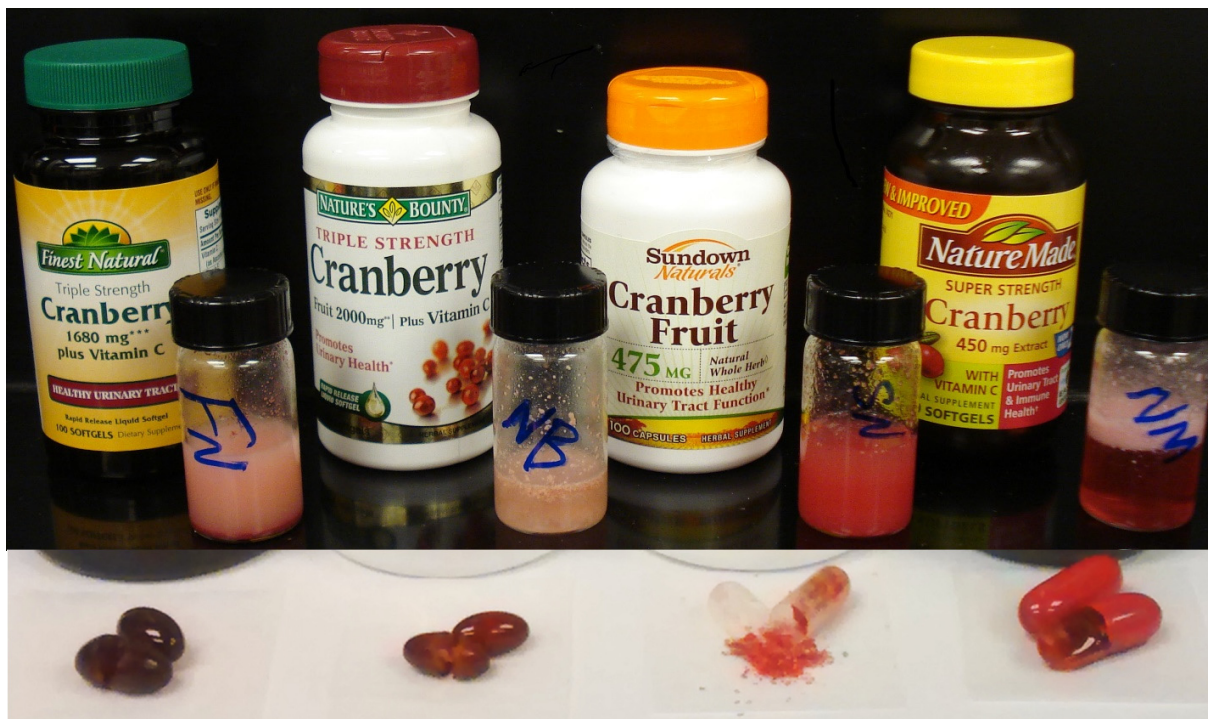
Figure 98. Cranberry dietary supplement products analyzed by HPLC-ELSC, showing packaging, labeling, capsules, and samples in aqueous solution. All four dietary supplement products resulted in aqueous solutions that had high amounts of insoluble material. These solutions were not similar to that obtained from cranberry juice powder (see Figure 99). These photographs were taken by C. M. Coleman on 2011-03-24.
