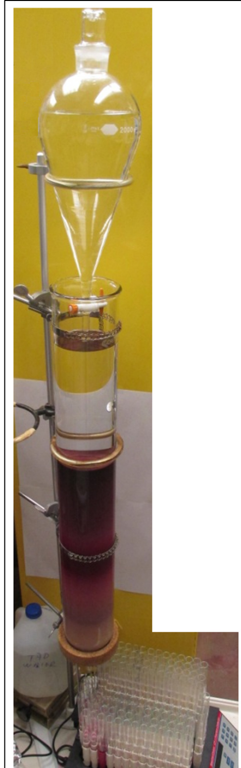
Figure 104. Overview of the configuration and equipment set-up for the CCA2 Sephadex LH-20 column.
