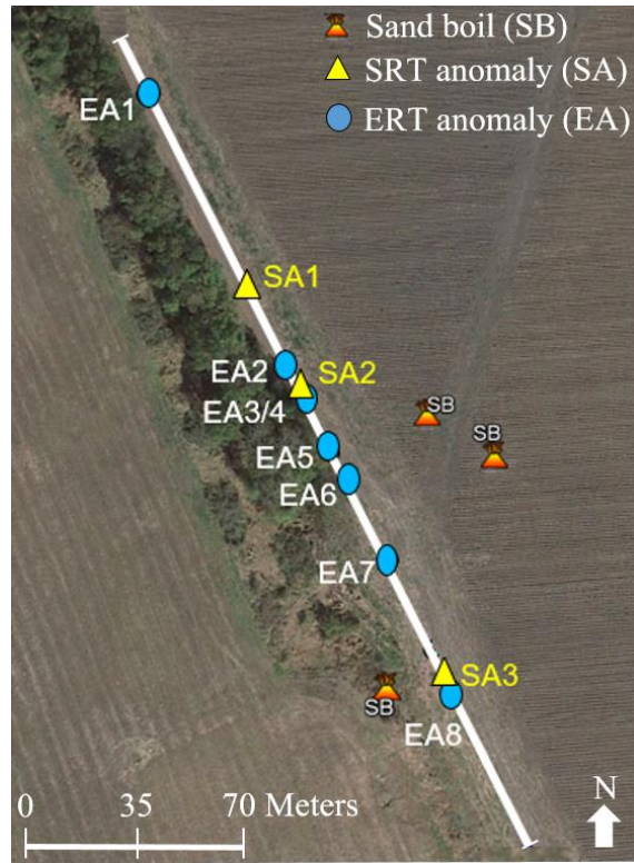
Figure 6.13: An aerial image of survey line 3 (landside) with locations of SRT and ERT anomalies indicated along the survey line.
