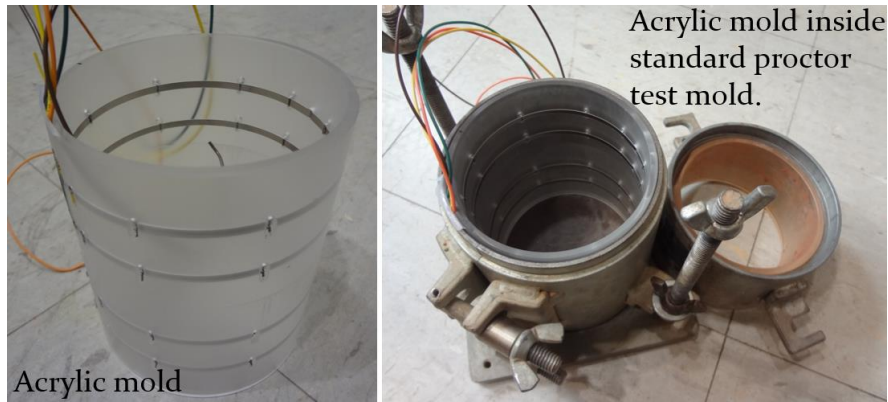
Figure 5.9: Acrylic mold with four electrodes.
