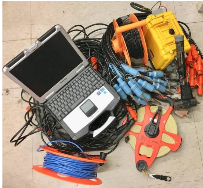
Figure 3.5: Equipment for seismic refraction survey.
