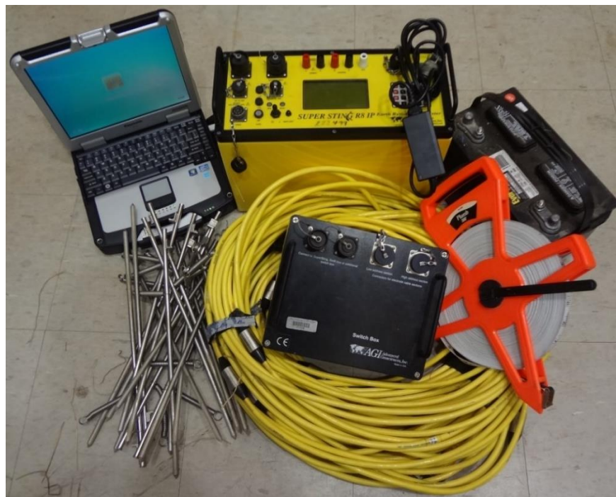
Figure 3.7: Equipment for electrical resistivity survey.
