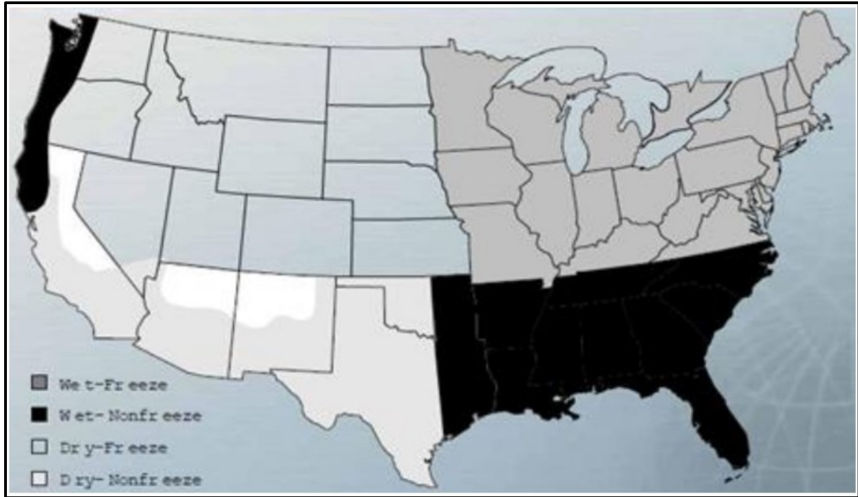
Figure 4. The initial climate zone map created during the LTPP test section recruitments [49]
