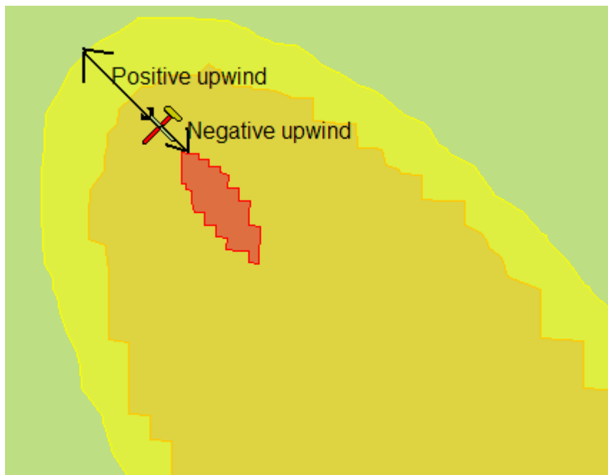
Figure C-9: Example of scenario when upwind distance is negative (plume zoomed in to origin)
