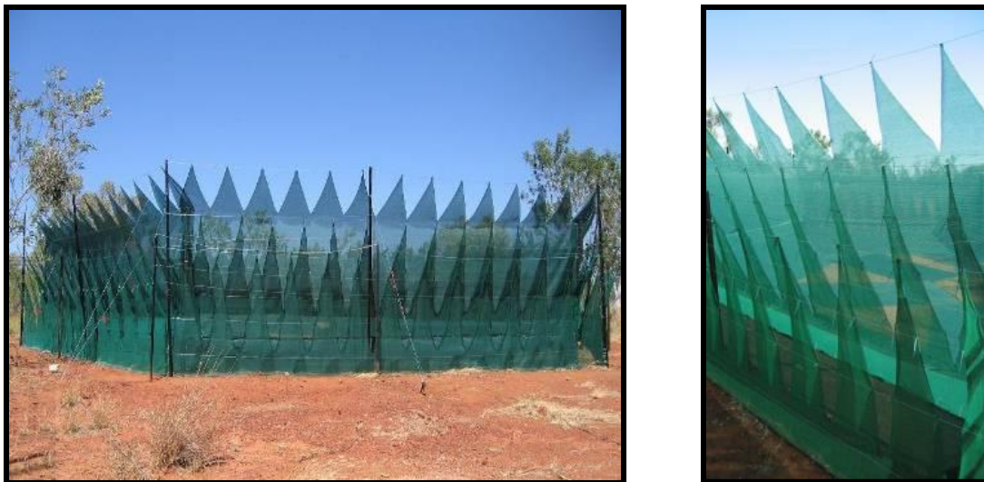
FIG. 10. Side and close up views of the fourth version of D. Christie turbulence-reduction enclosure. Structure is made of porous fence material, and multi-walled, with serrated outwardly pointing walls. (Pictures taken from presentation by D. ReVelle 50 )
