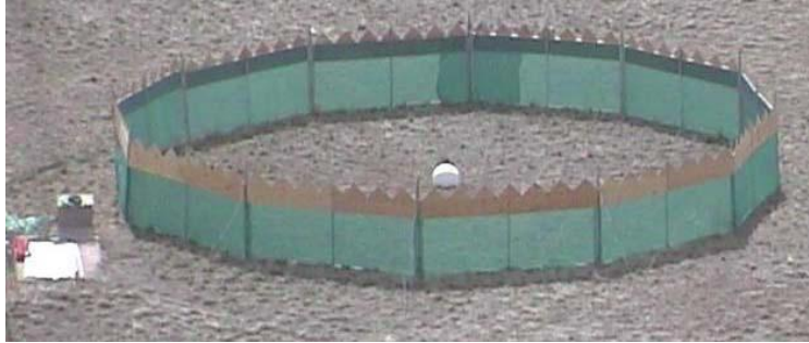
FIG. 8. Turbulence-reduction device designed and used by A. Bedard and NOAA for tornado detection. A micro-barometer is located at the center of the structure. The structure is 15.25 m in diameter and 1.8 m in height, and covered in green porous fencing material. (Picture taken from Bedard et al. 52 )
