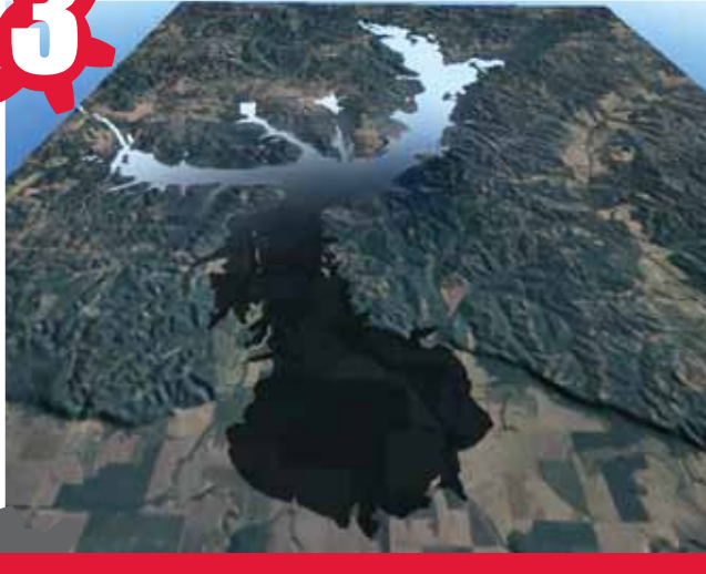
Animation of the hypothetical breaching of Arkabutla Dam, MS, created by simulation software DSS-WISE Lite.
