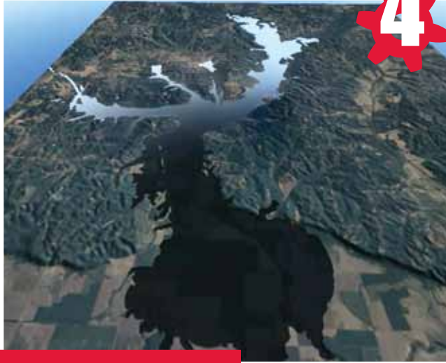
Animation of the hypothetical breaching of Arkabutla Dam, MS, created by simulation software DSS-WISE Lite.
