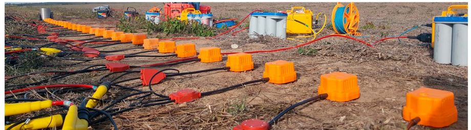
Figure 3. Experiment setup with shaker and geophone array.
