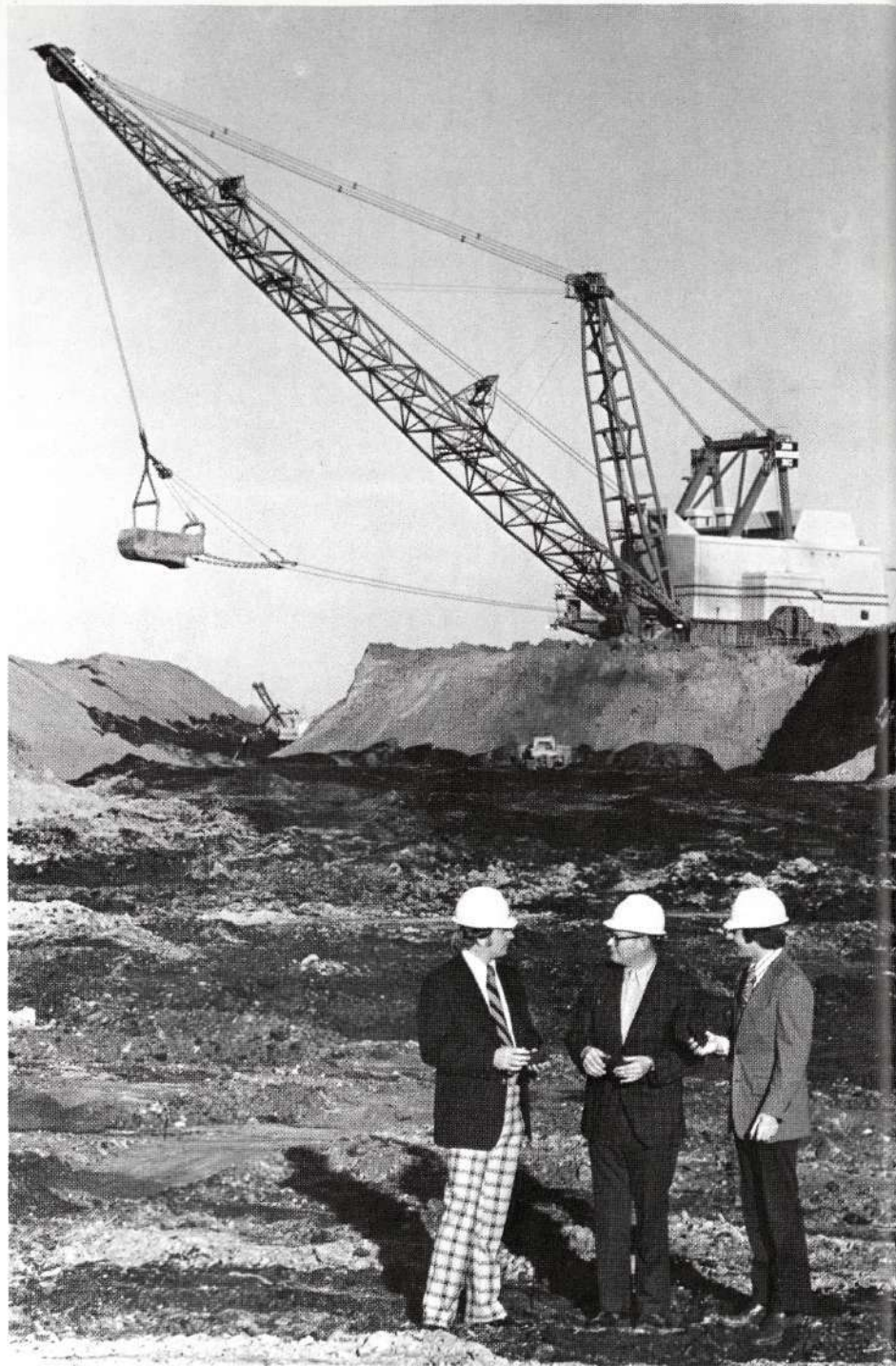
Dragline. Seniors Bill Peck ( l. ) and Julian McNeely ( r. ) examine chunks of lignite, a form of soft coal, with Harold Williamson, manager of accounting and purchasing for the Big Brown Steam Electric Station. The massive dragline, which dwarfs the bulldozer working below in the pit, removes overburden in 70-cubic-yard bites. After the lignite is removed, the earth is redistributed, topsoil is restored and trees, grasses and native vegetation are planted.
