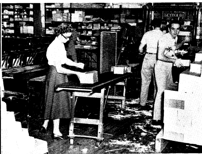
6. Journals rolling from binding machine onto trimmer which evens the edges of pages; then stacked on skids for mailing.
