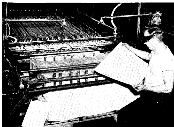
5. Pressman examines a 32-page sheet as it slides off one of the huge presses which print about 1,000 Journals an hour.
