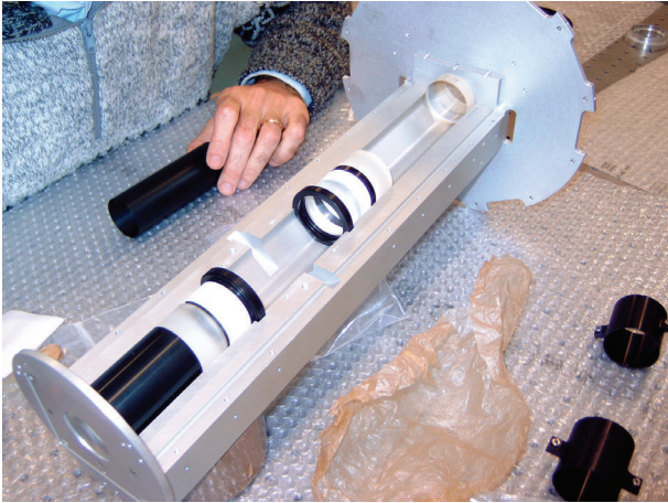
FIGURE 6: Assembling of lenses and spacers on the V-cave of the optical bench.
