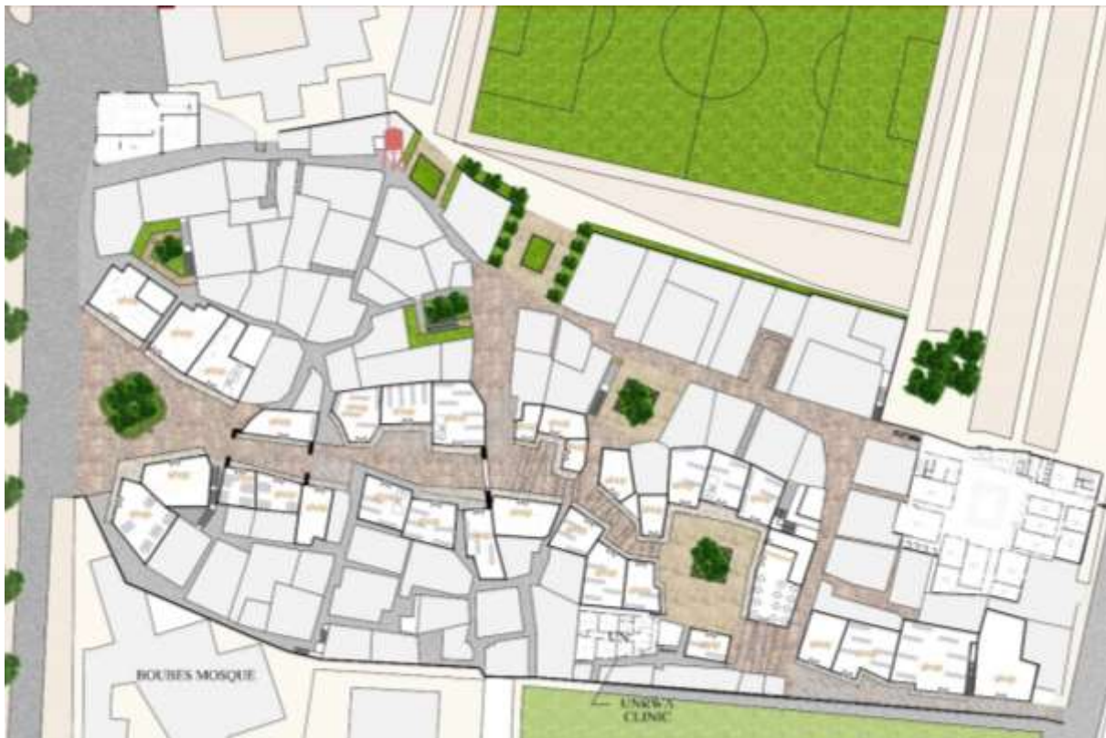
Fig.14: Ground Floor Plan showing the shops and the circulation walkway path, after the intervention
