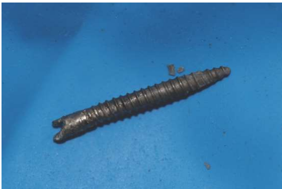
Fig.2h: Removed post with remnants of cement around it. Reference: The authors - April 2019
