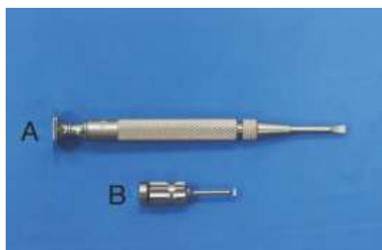
Fig.1: A jewelers' precision stainless steel flat-blade screwdriver. B; Manual flat-blade abutment driver.
