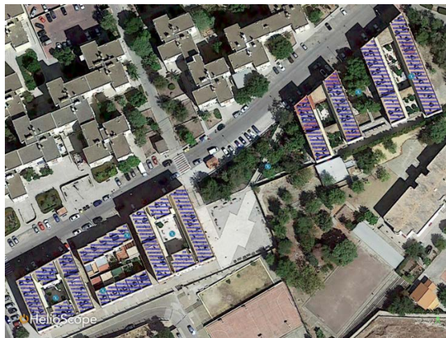
Figure 11: Example of layout of the district in Helioscope: south orientation in the flat roofs.
