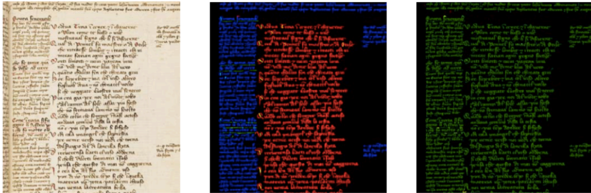
Figure 13 - Example of layout analysis on the DIVA-HisDB test. On the left the original manuscript image, in the middle the classes pixel-wise labelled by the DhSegment and on the right the comparison with the ground-truth. Adapted from [14], p. 11, ©2018 IEEE
