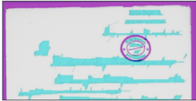
Figure 15 - Piece of an image displaying tight ("glued") regions of text with a covering displayed in cyan color as well as coverings of marginalia, separators and graphics displayed in magenta. Adapted from [12], p. 268, ©2018 IEEE.
