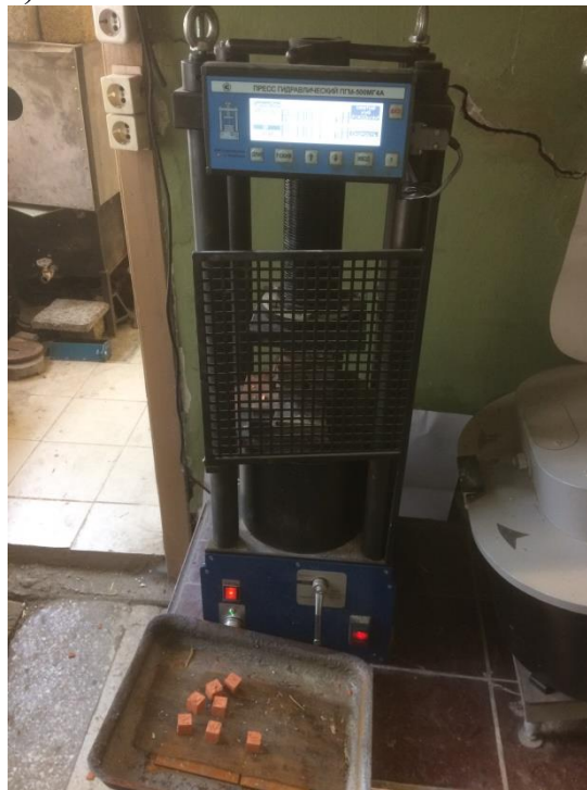
Figure 3.2. - Testing of ceramic samples in the press SGP - 500MG4A
