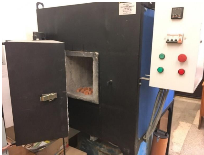
Figure 3.1. - Furnace chamber, model PKC-30 / 12.5
