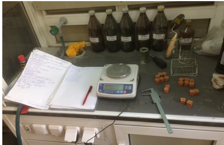
Figure 3.4. - Workplace in the determination of shrinkage
