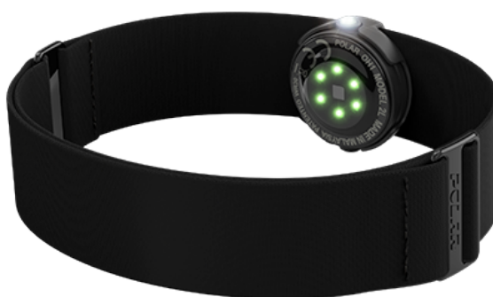
Figure 3.10: Polar OH1 armband – a 6-LED optical HR sensor.
