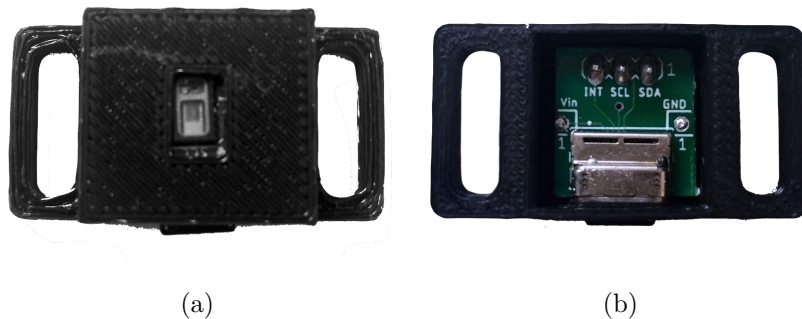
Figure 7.2: Setup: (a) 3D-printed black box front; (b) 3D-printed black box back.
