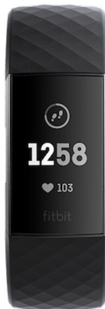
Figure 3.9: Fitbit Charge 3 face displaying the time and the user's heartbeat.
