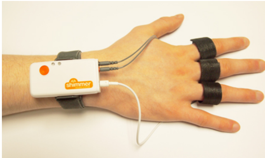
Figure 3.5: A user's hand with Shimmer3 GSR collecting vital signs as PPG [2].
