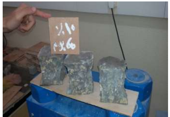
Figure 5: Failure Mode of concrete specimens with 10% of glass powder after 60 days
