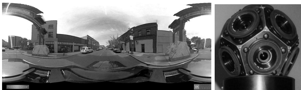
Figure 2-2 Onnidirectional camera and a corresponding spherical view.[5]
