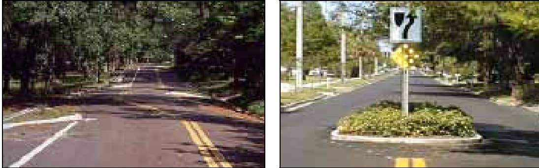
Figure (53) Traffic Calming - Narrowing
