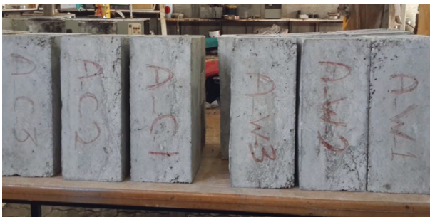
FIGURE 11: The A-B jacketed column specimens ready for testing.
