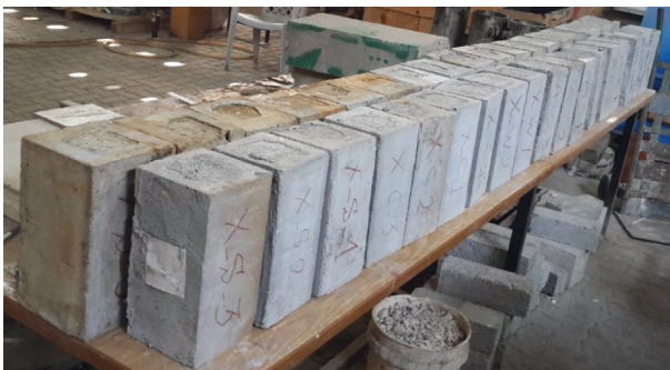
FIGURE 12: The X-Y jacketed column specimens ready for testing.
