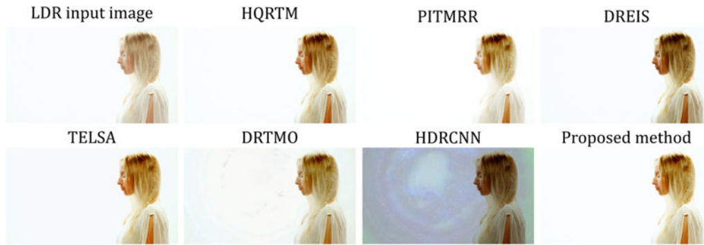
Fig. 9. Comparison of different results obtained by each tested algorithm using a highly overexposed image as input. As can be seen, DRTMO and HDRCNN produce artifacts in overexposed areas. For visualization, HDR images were tone-mapped by Mantiuk et al. [39] operator.
