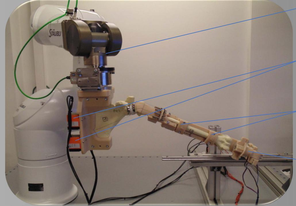
6-DOF robot for active control of the humeroscapular joint
