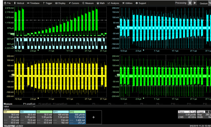
Figure 4.34: Top left: i_{PD} as measured with reference photodetector, and internally generated SOB signal (measured through v_{CMLM} ). Bottom left: v_{OD} with the LBMRX operating in burst mode, but with fixed gain. Top right: feedforward AGC only. Bottom right: feedforward + feedback AGC.
