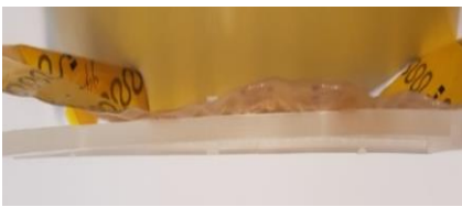
Figure 7: Over-molded flexible electronics foil with PP
