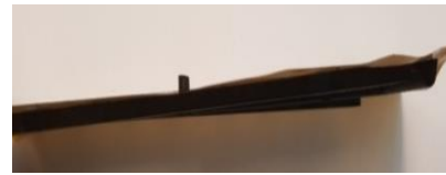
Figure 10: Over-molded flexible electronics foil with GF-PA6.
