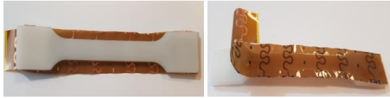
Figure 6: A trimmed over-molded flexible electronic circuit for peel test
