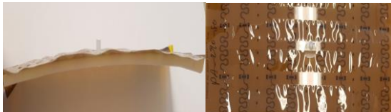
Figure 9: Over-molded flexible electronics foil with PA6.
