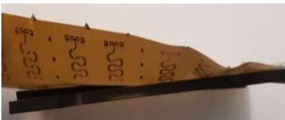
Figure 8: Over-molded flexible electronics foil with GF-PP.
