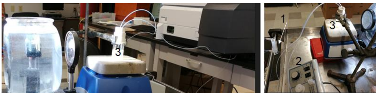
Figure 2.2 In-situ diffuse reflectance spectroscopy set up 1: flow-through cuvette 2: mini-pump 3: reaction vial
