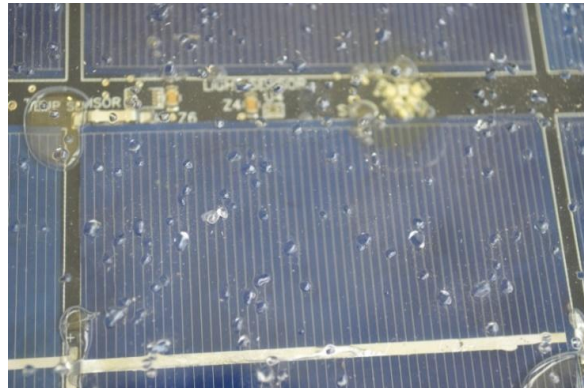
Figure 7. Example Panel Variations due to Manufacturing Process (i.e., Internal in-Polymer “Bubble” Formation)
