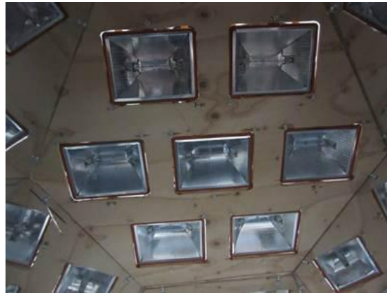
Figure 8. Photograph of the Solar Roadway Panel Solar Tester
