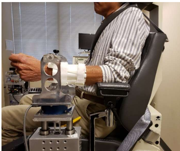
Figure 2.1. Experimental Setup for Elbow Force Measurement.
