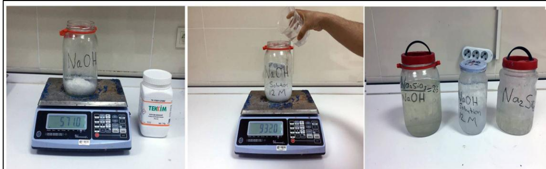
Figure 3.1 Preparing alkaline activator
