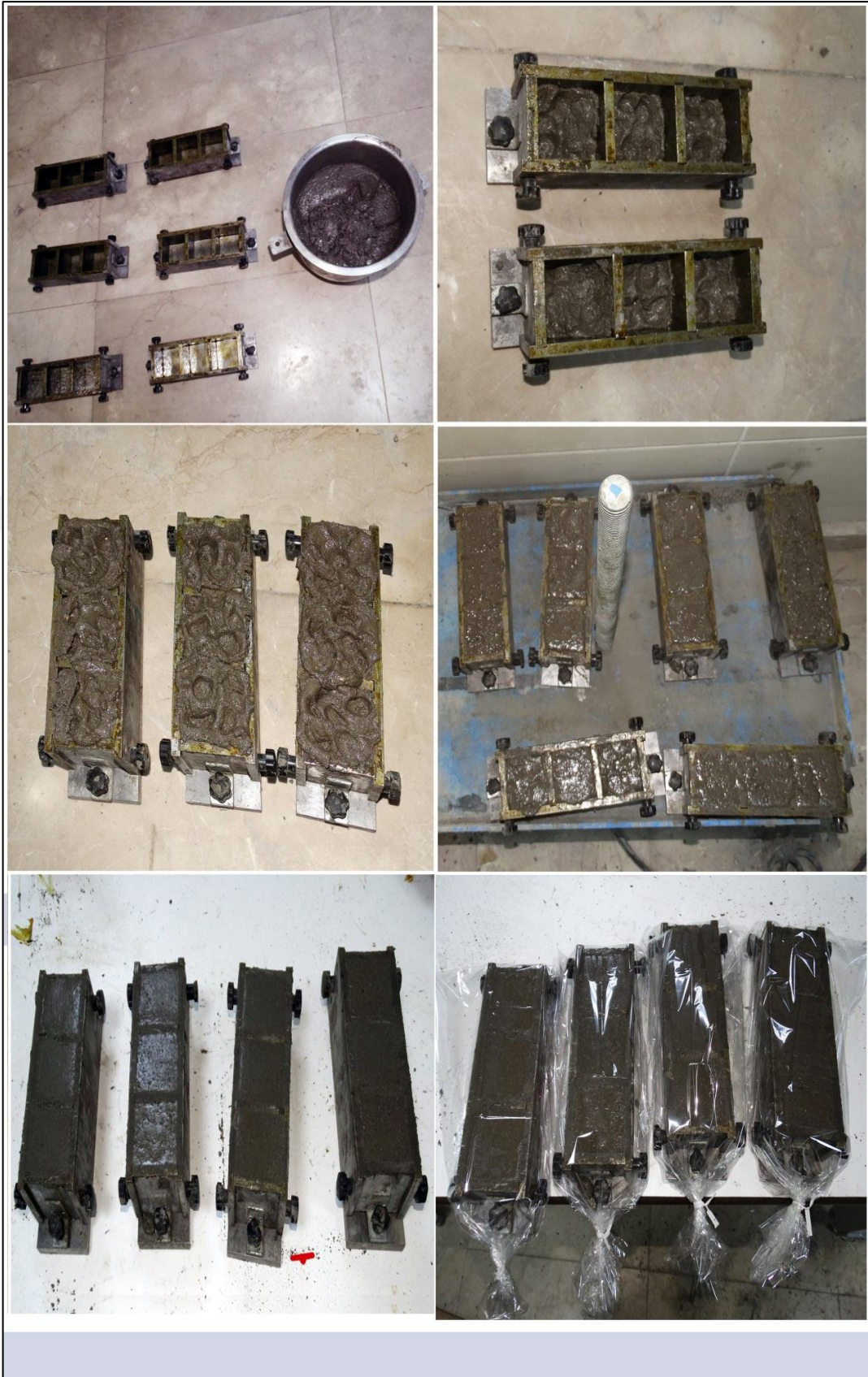
Figure 3.6 Casting geopolymer mortars
