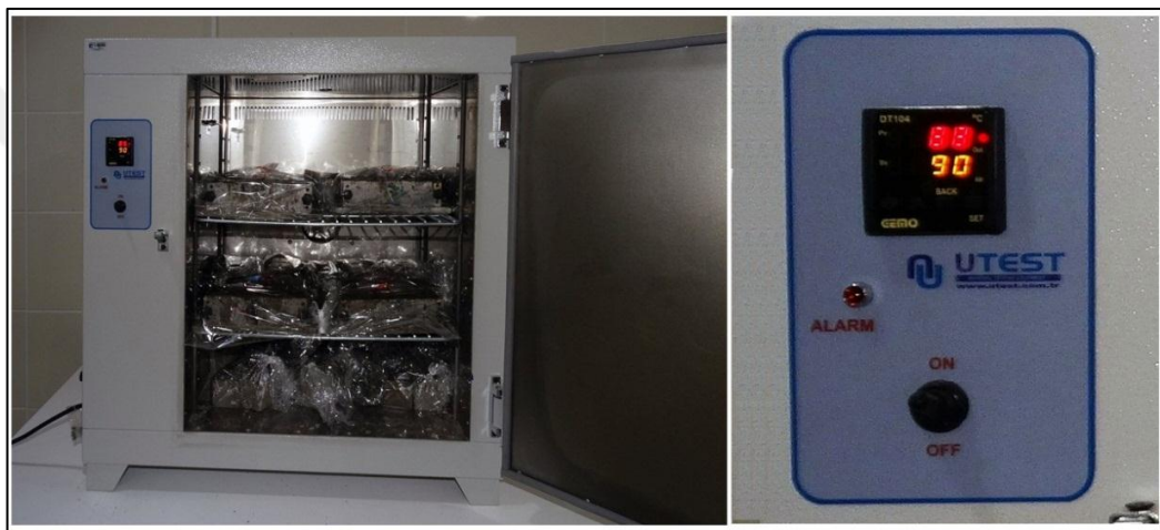
Figure 3.7 Curing cubic specimens by oven dry
