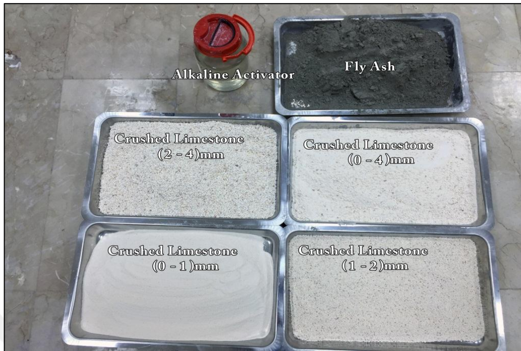
Figure 3.3 Preparing geopolymer mortar constituents
