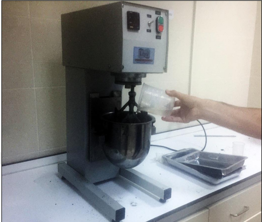
Figure 3.5 Adding alkaline activator to the dry components
