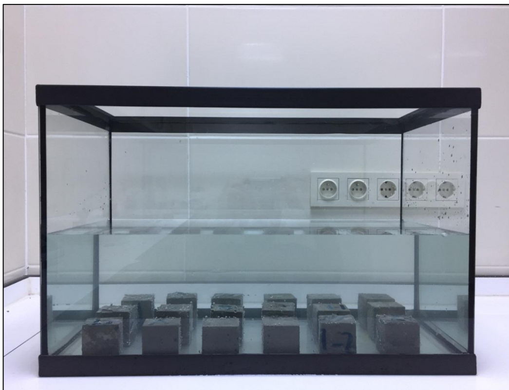
Figure 3.10 Water absorption test by total immersion
