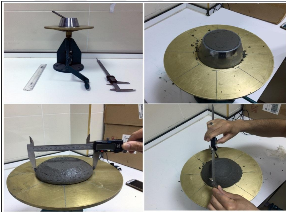
Figure 3.8 Flow table test of geopolymer mortar
