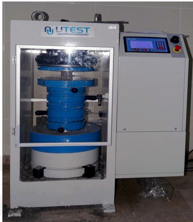
Figure 3.9 Compressive strength test
