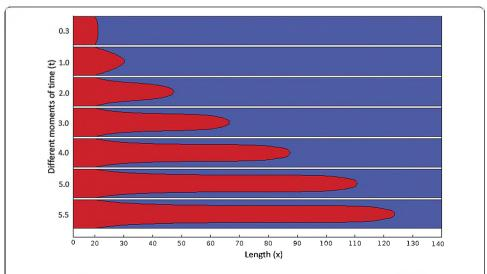
**Figure 1 Numerical simulation: successive positions of the free boundary in a single capillary.** Due to the boundary condition (18), the contact points of the free boundary and the solid skeleton will be permanently fixed at the initial position. Numerical implementations predict the appearance of a water tongue, which grows with time.
