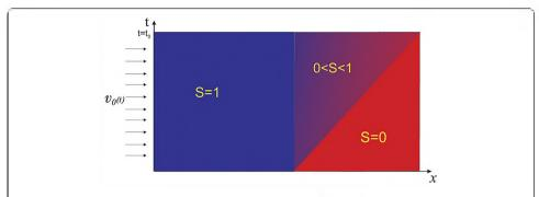
**Figure 4** The limit of rigorous numerical upscaling. The domain occupied by the water tongues at a fixed time becomes under homogenization a mushy region, where the concentration s of water varies from 1 to 0.
