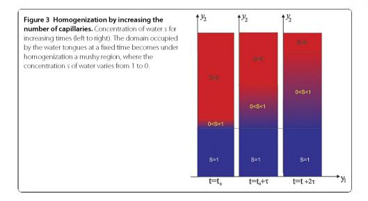
gradual growth of the number of capillaries (Figure 2) leads to homogenization of the liquid motion. The domain occupied by the water tongues at a fixed time becomes under homogenization a mushy region, where the concentration *s* of water varies from 1 to 0 (Figures 3 and 4).
