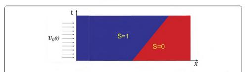
Figure 5 The solution of the Muskat problem. The free boundary separates two liquids and moves with a constant velocity.
