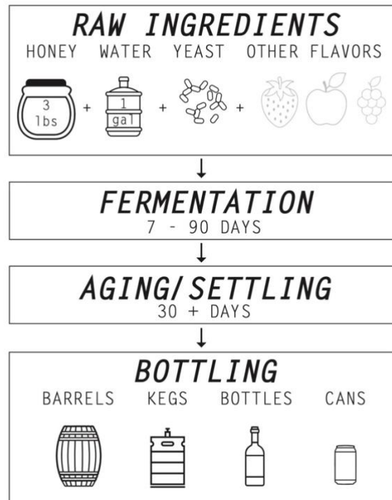
Figure 15 Mead Brewing Process Overview, drawing by author.
