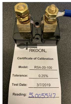
Figure 3.19: 0.005 \Omega shunt resistor and calibration certificate, used to sense current in the low voltage AC power analyzer.
