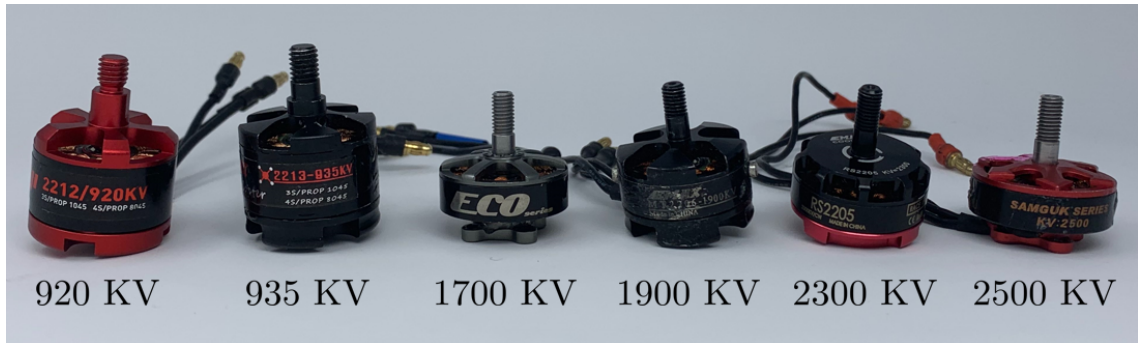
Figure 5.1: BLDC motors tested using the custom dynamometer.
