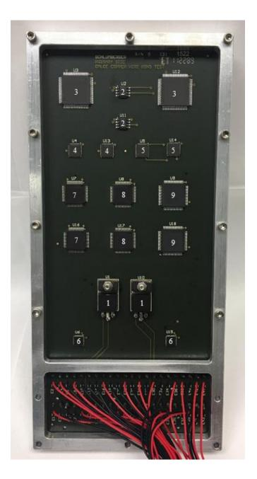
Figure 3.3: Printed wiring assembly with Al frames on both sides.
