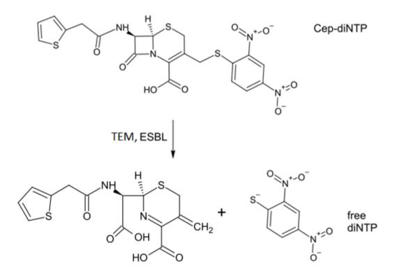
Figure 5.4. Cep-diNTP substrate can be hydrolyzed by both a non-ESBL classical  $\beta$ -lactamase (TEM-1) and ESBL.
