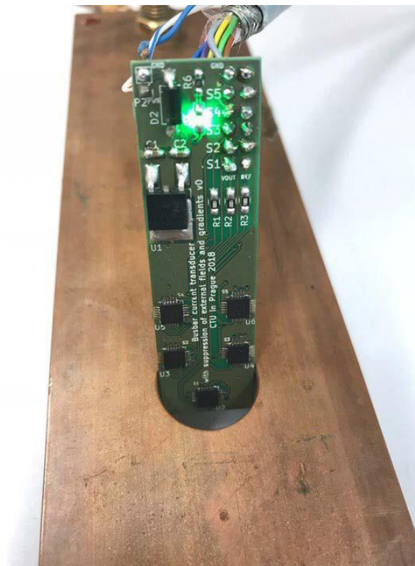
Fig. 10 High current transducer with 5 microfluxgate sensors inside the busbar [79]
