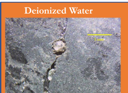
Induced fractures and impingement in wet core w/ CT cross section
