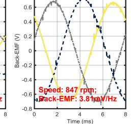
Comparison of line-to-line open circuit voltage of all 3D printed motor (image shown below) with bonded magnets (left) and sintered NdFeB magnets (right)
