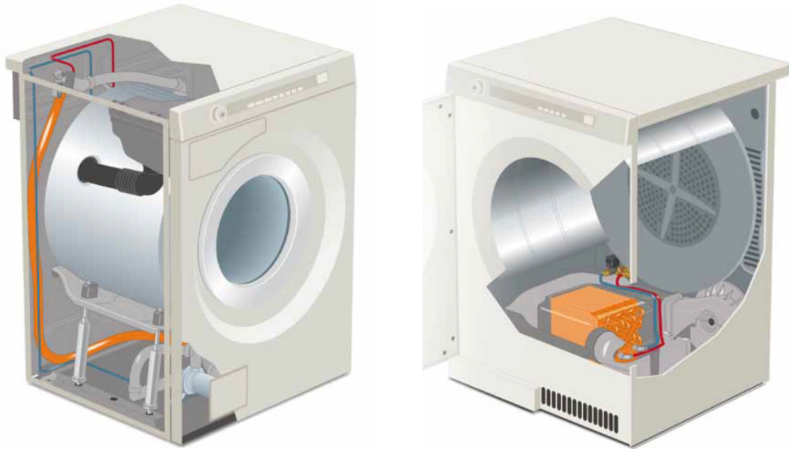
Figure 5.3 Heat fed washing machine and clothes dryer from ASKO® with built-in water-to-water and water-to-air heat exchangers, respectively (in orange)
