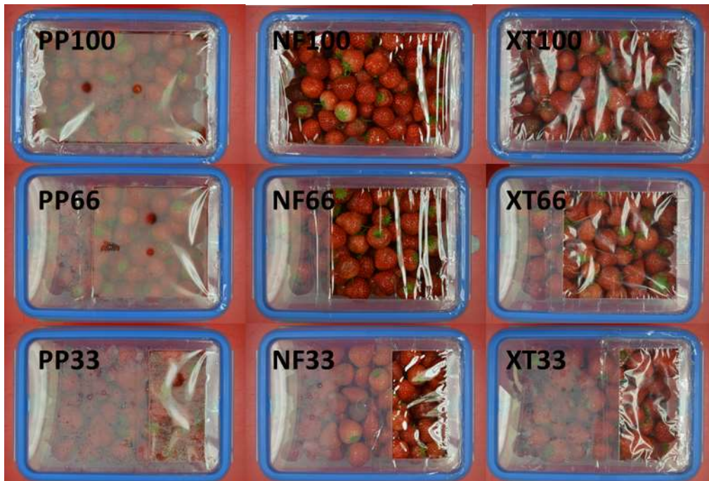
Figure 2. Visual documentation of lid and film condensation after 14 days of storage.
