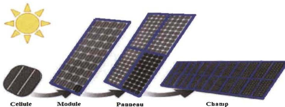
Figure 1.3. Configuration des cellules photovoltaïques [38]
