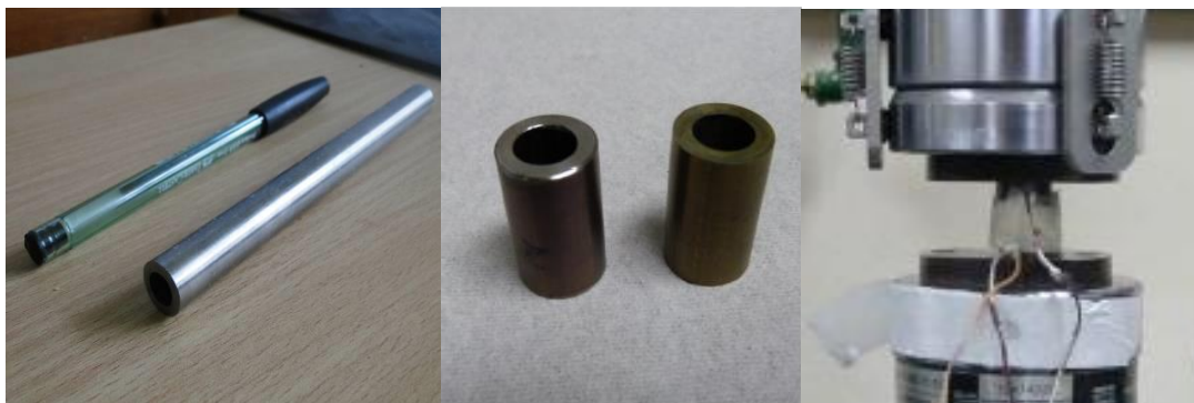
Figure 3: NiTi SMA utilized for the fabrication of the actuators. a) Bar in its received condition. b) Two NiTi hubs subjected to different thermal treatments. c) NiTi hub with the coiled electric heater ready for a compression test for the activation procedure in the MTS 810 machine.
