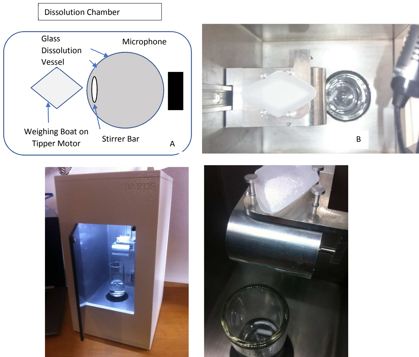
Figure 2: (A) Top view schematic diagram representing the contents of the dissolution chamber and (B) photograph of the BARDS dissolution chamber. Note the microphone is not in contact with the vessel. External view of the instrument (C) Tipper motor with a sample in a weighing boat ready for addition to the stirring solution below.
