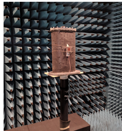
Fig. 17: Anechoic phantom mounted off-body far field pattern measurement setup.
