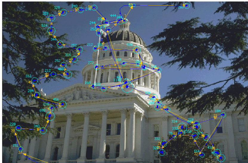
Figure 2.8: An example of a scan path over an image. Light blue circles indicate fixations with diameter proportional to duration of the fixation, yellow arrow indicate the saccades and the blue path is the actual movement of the gaze point. Image obtained with SR Research Data Viewer https://www.sr-research.com/data-viewer/
