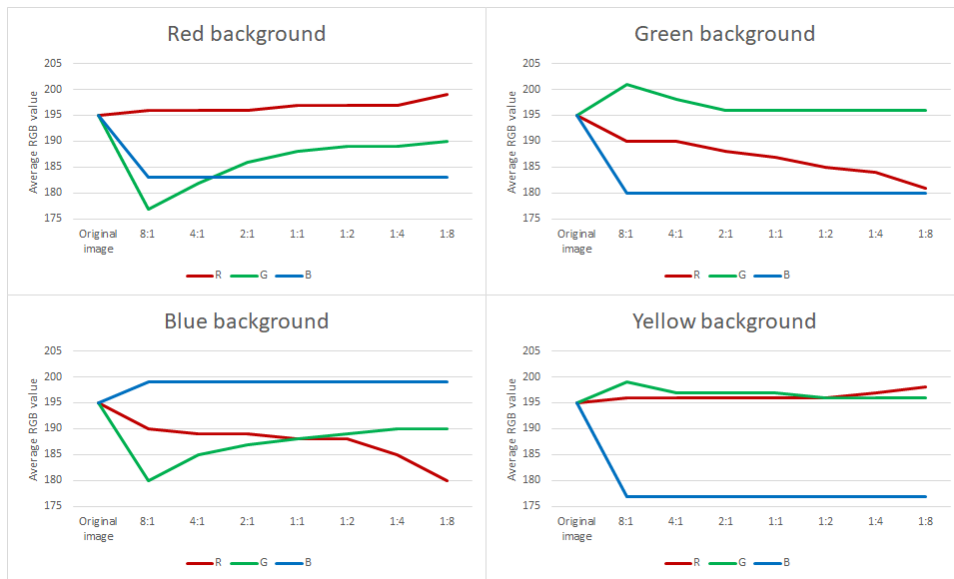
Figure 7.15: Average RGB value for each channel for the four squares with different colored backgrounds of Table 7.5, with varying L:M cone ratio.
