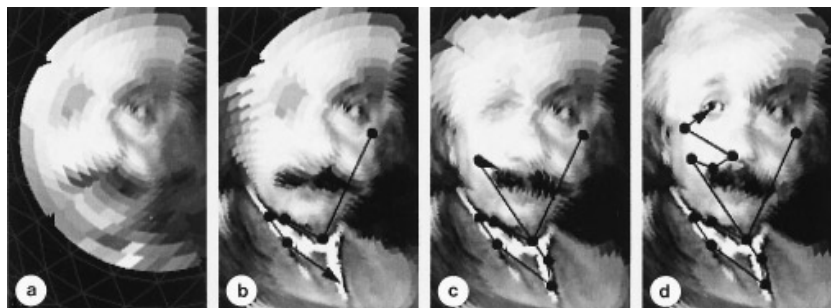
Figure 3.3: Simulation of a gaze movement pattern with an active foveated vision system, exploring a grayscale image of Einstein. Image courtesy of [69].
