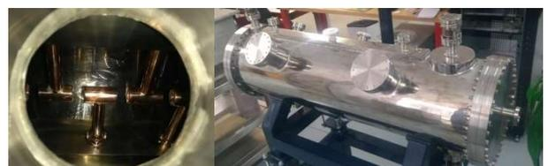
Figure 3. IH cavity prototype.
