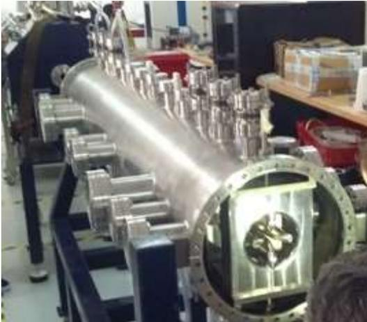
Figure 2. The four-vane RFQ
