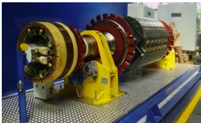
Figure 5.2: Example of manufactured salient-pole solid rotor (courtesy of Nidec-ASI, Monfalcone, Italy)
