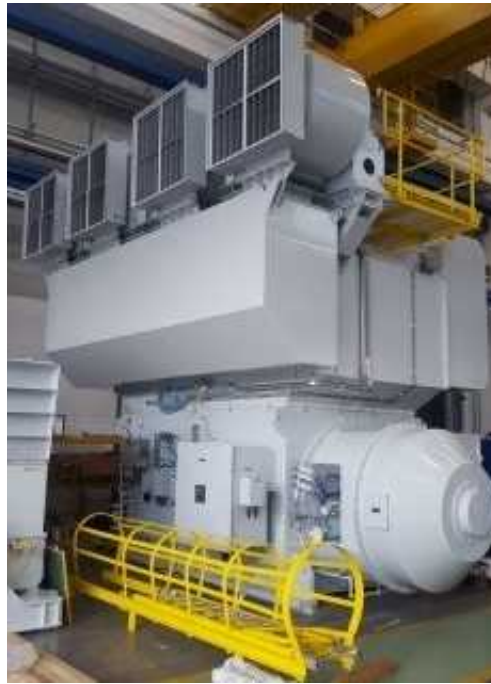
Figure 8.4: Synchronous motor with DOL-starting capability (courtesy of Nidec-ASI, Monfalcone, Italy)
