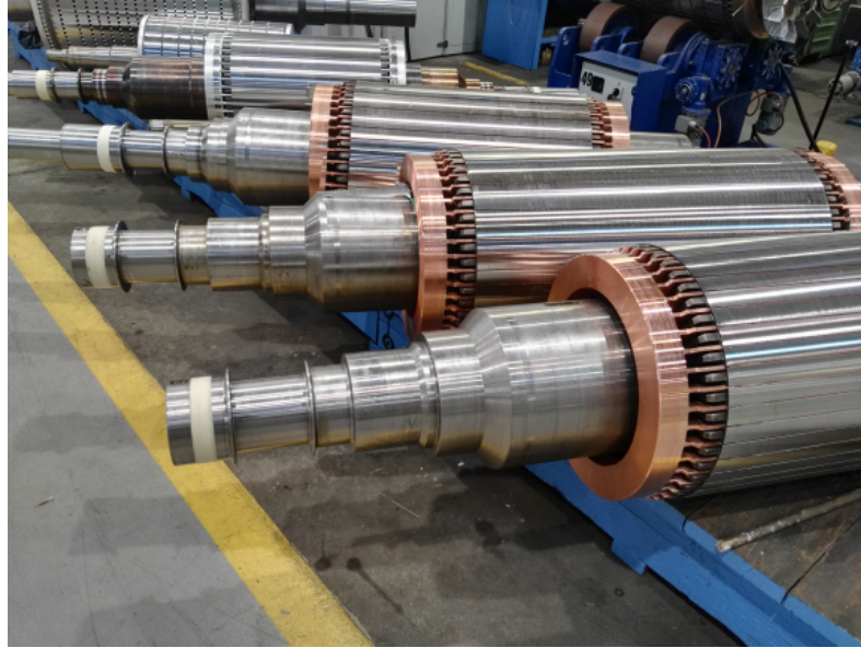
Figure 1.1: Rotors of MV two-pole squirrel-cage IMs with laminated core and solid-steel shaft (courtesy of Nidec ASI, Monfalcone, Italy)
