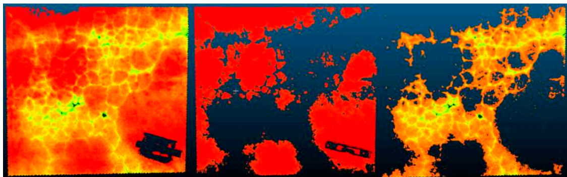
Figure 27. Segmentation of pavement section 3 with RANSAC.
