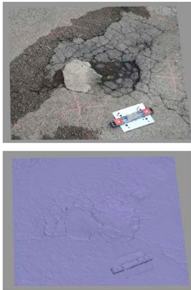
Figure 11. Model of distress 2—(top) and dense cloud—(bottom) produced by imagery from Samsung Galaxy s9.
