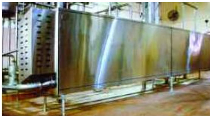
Fig. 2-6. Heat exchanger made of duplex stainless steel grades.
