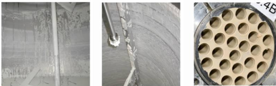
Fig. 2-11. Visual appearance of a tank filled with yogurt (first two pictures on the left) and of a tubular heat exchanger in a UHT plant that has been heating white milk at 120°C (last picture on the right) 81 .
