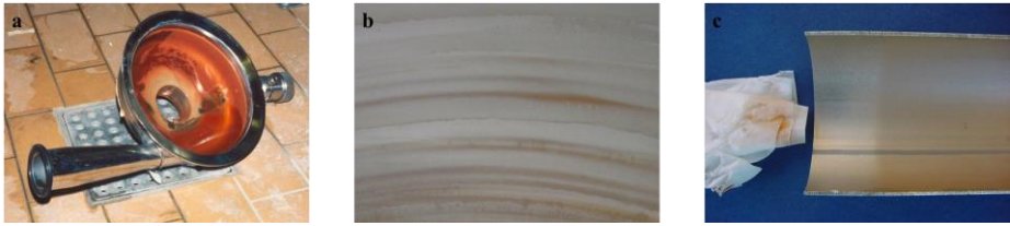
Fig. 2-7. Rouging build-up on a) the house pump b) in the buffer tank in the storage section and c) in piping through movement equipment 53 .
