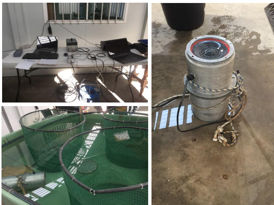
Fig. 50 Acoustic emission system. At the top left are the systems for acoustic emission and video recording. Lower left the emitter inside the tank and the baskets where the fish were placed. On the right the acoustic emitter.
