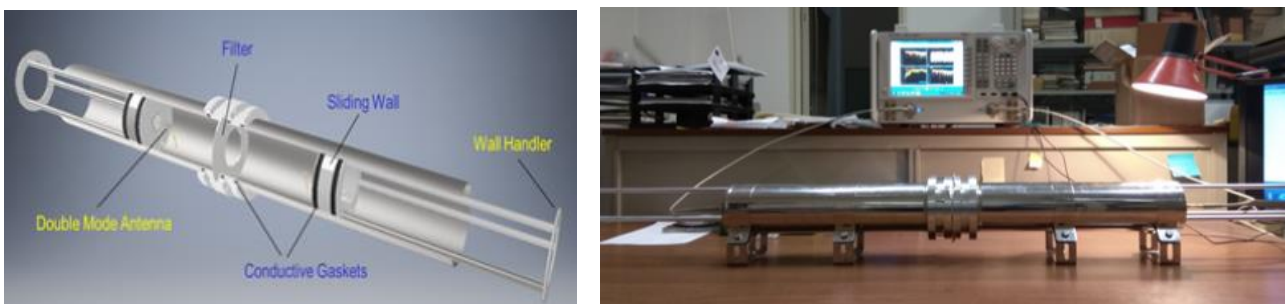
Figure 5.9 - High frequency band ( 2 \div 20 GHz) test setup: schematic (left); photo (right).
