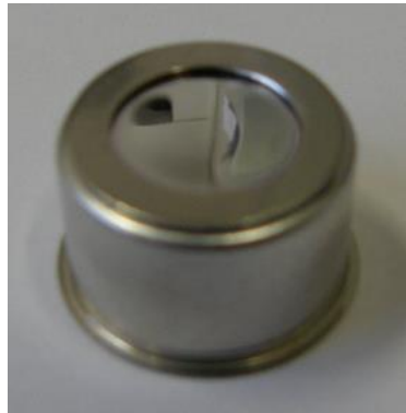
Figure 5.4 - C2-1 filter mounted on a TO8 frame. The clean aperture of the filter is 8 mm.
