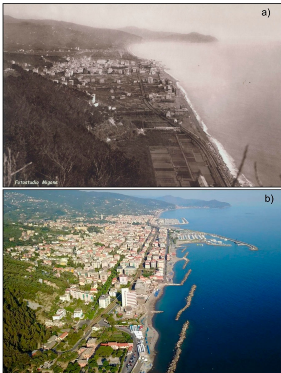
Figure 3. The floodplain and shoreline modification over the last two centuries: (a) view of Chiavari and Lavagna in 1890 ('E. Migone', photographer archive in Chiavari); (b) recent view of the urbanized floodplain and modified shoreline (P. Giacomelli).
